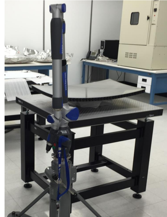
Portable CMM in small clean room with mirror prepped on optical table for measurement
